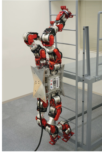
FIGURE 2.4: WAREC-1 is designed as a search and rescue robot and has the capability to climb as one of its locomotive styles [26, 41]
