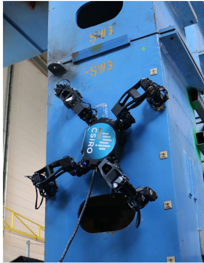
FIGURE 2.6: Magneto has magnetic feet and is designed for cluttered vertical environments [17].
