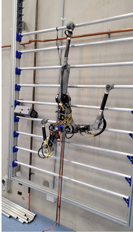
FIGURE 7.1: The ParCli robot passively perching on a vertical ladder
