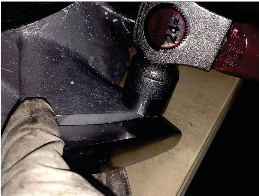
Figure 106 – Repair of damaged vane tips
