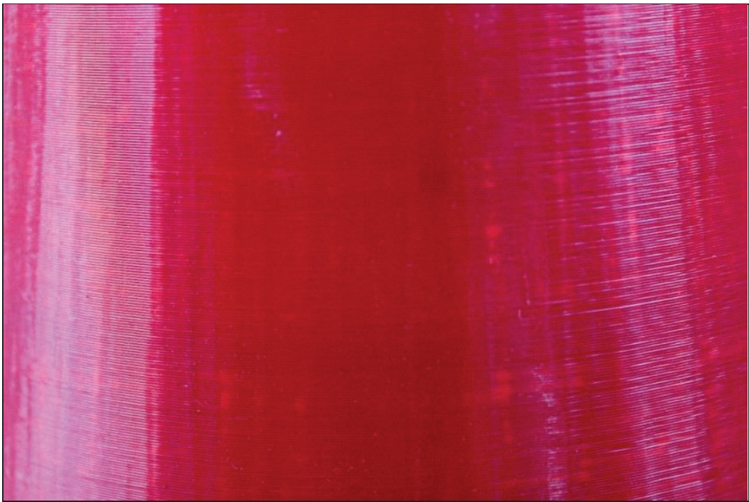
Figure 97 – 3D print surface before sanding
