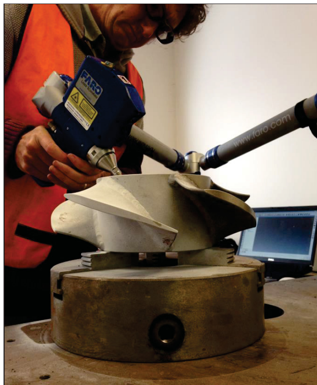
Figure 46 – CMM measurement of new impeller
