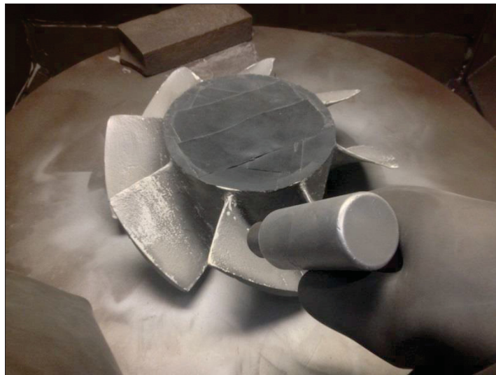
Figure 104 – Bead blasting the impeller to remove paint.
