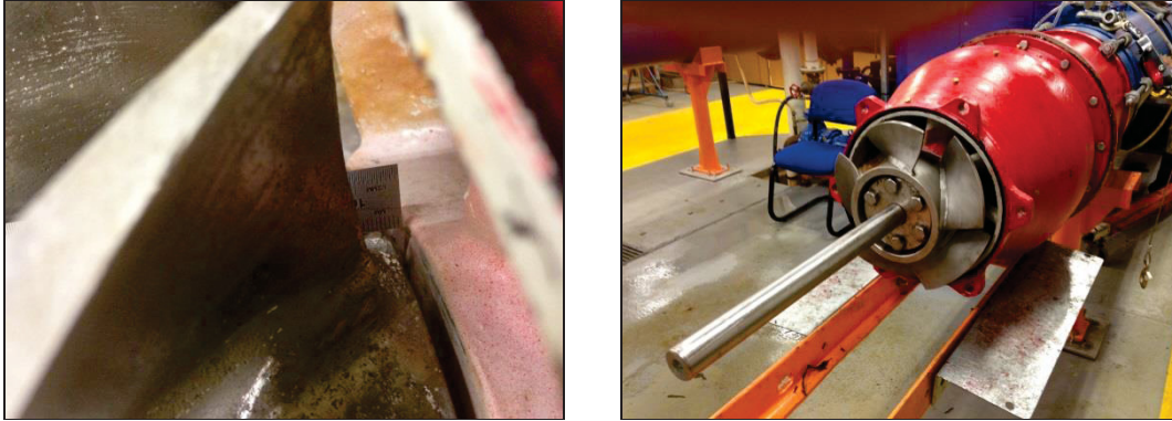
Figure 196 – Impeller running gap check, new diffuser installation
