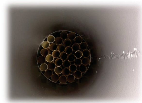
Figure 172 – Pipe internals showing straightener section
