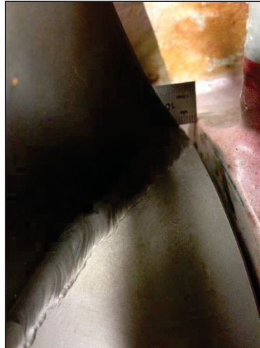
Figure 203 – Impeller running gap check for five vane impeller
