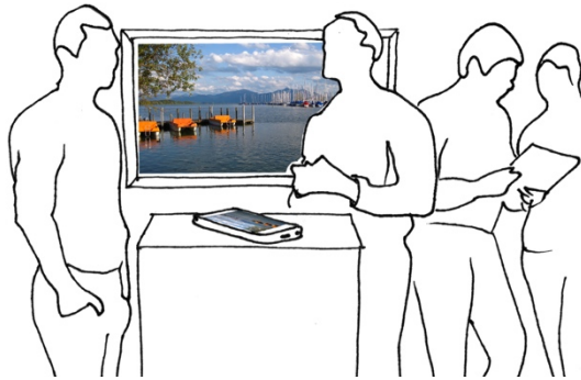
Figure 5: C3. Single Share , a smartphone showing the relevant photo is placed on top of a special dock, and the content is instantly displayed on a large screen
