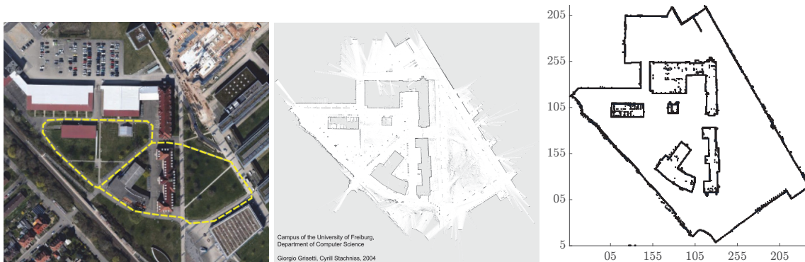
FIGURE 5.6: The left picture shows the satellite map of the Freiburg University Campus where the yellow dashed line indicate the robot trajectory. The middle figure shows the corresponding occupancy map of the dataset (Howard and Roy 2003). The right figure shows the corresponding binary map of obstacles used for exploration experiments. Map dimensions are in meters.
