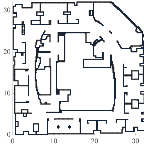
FIGURE 5.3: The constructed environment for exploration experiments using the binary map of obstacles from the Intel dataset.
