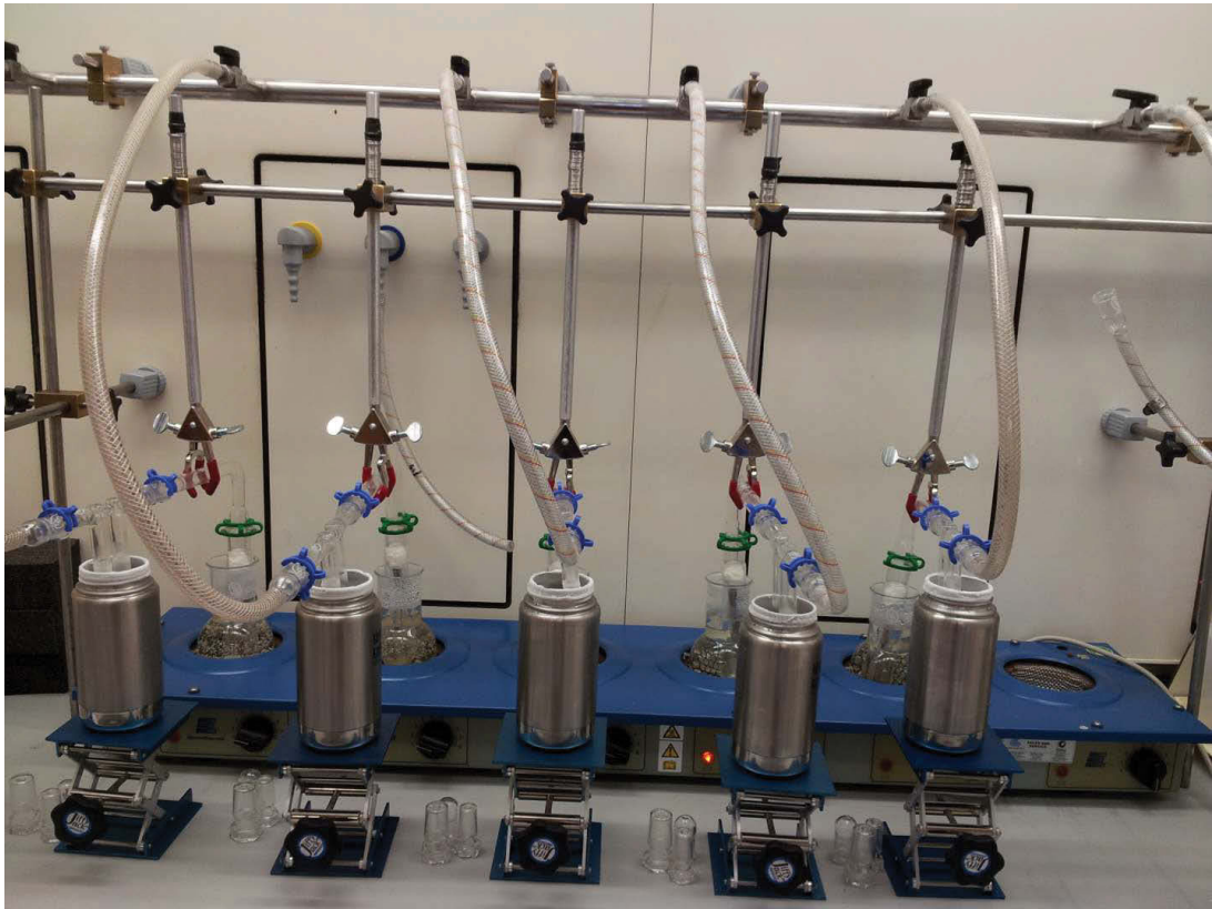
Figure 2.1: Cryogenic distillation system to extract water for stable isotope analysis.
