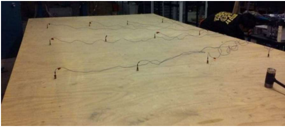
Figure 10: Photo of the experimental arrangement with the 12 sensors and impact hammer.
