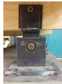
Figure 7: Photo of the pin support of the ribbed deck floor.
