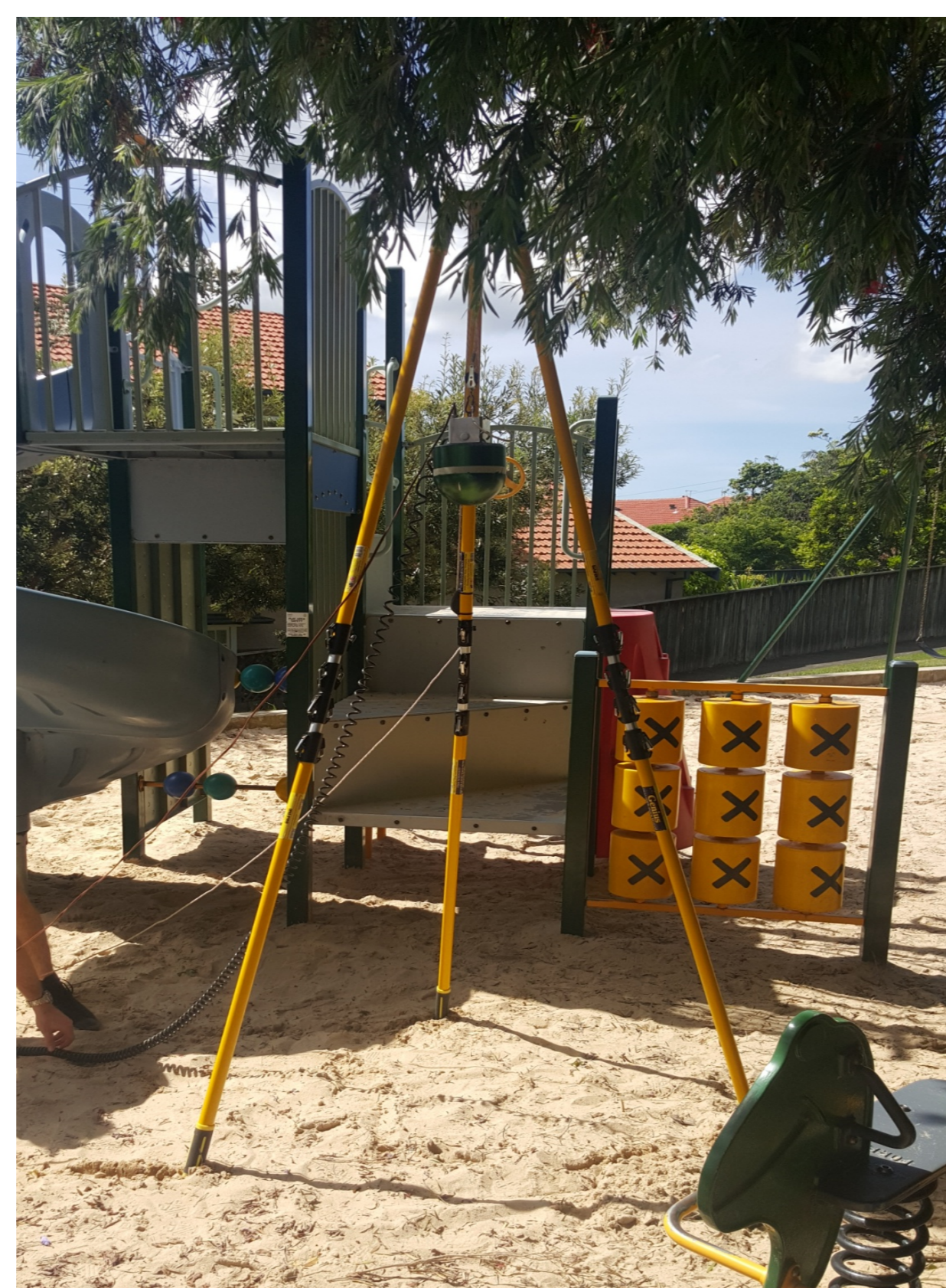
Figure 3: Drop test set up at Reginald St Park Mosman
