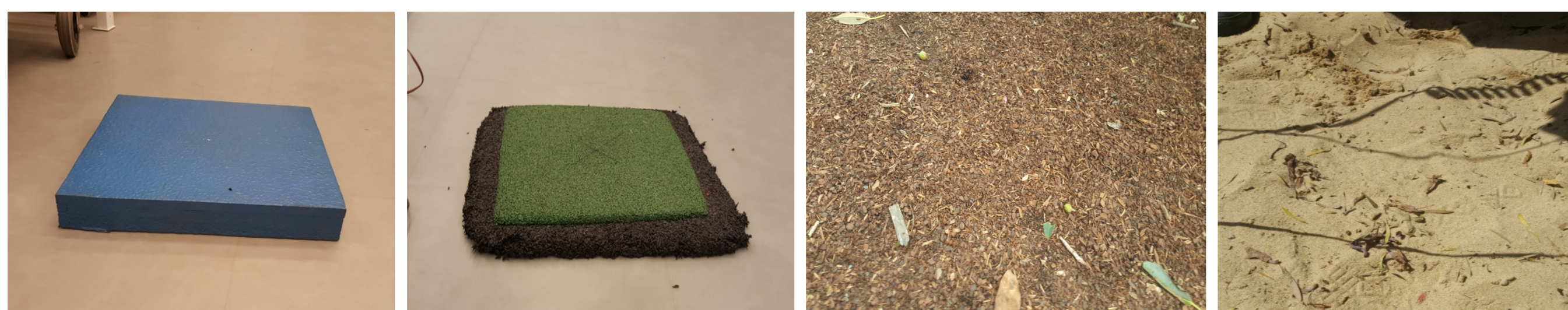
Figure 1: Impact attenuating surface materials. Left to right: thick rubber, thin rubber, bark and sand
