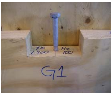
Fig. 2 Notched coach screw connection detail
