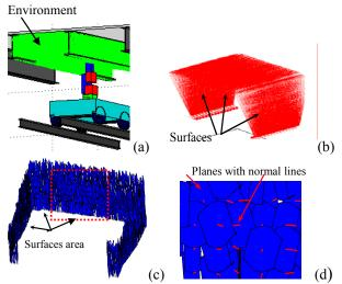
Figure 3 (a) Blasting environment; (b) Surfaces; (c) Surfaces and small blasting area; (d) Small planes with normal lines
