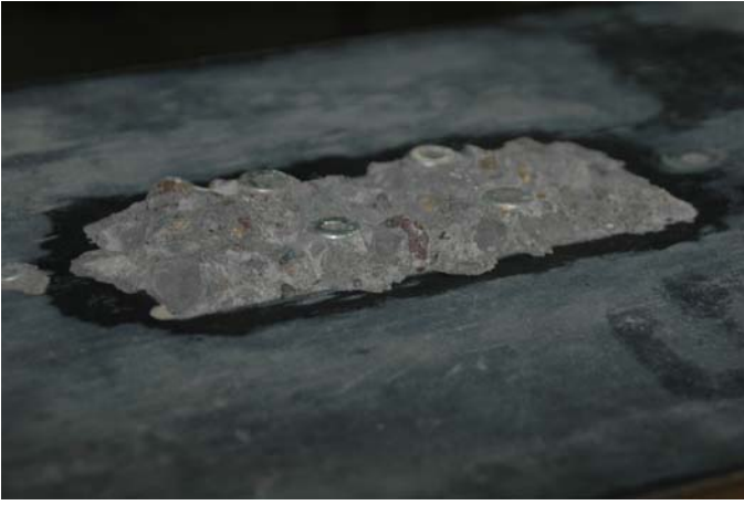
Figure 7: Failure of a specimen with wood screws.
