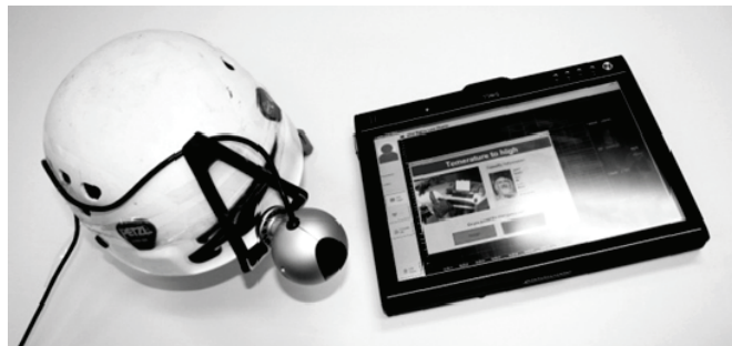
Figure 6. Helmet with mounted webcam and Dell Latitude XT tablet PC
