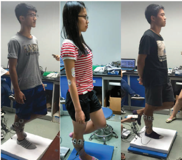
Fig. 2. The three scenarios of one-leg standing subjects during experiment. From left to right: T1 (proprioceptive senses lost); T5 (vision lost); T2 (proprioceptive senses and vision lost).
