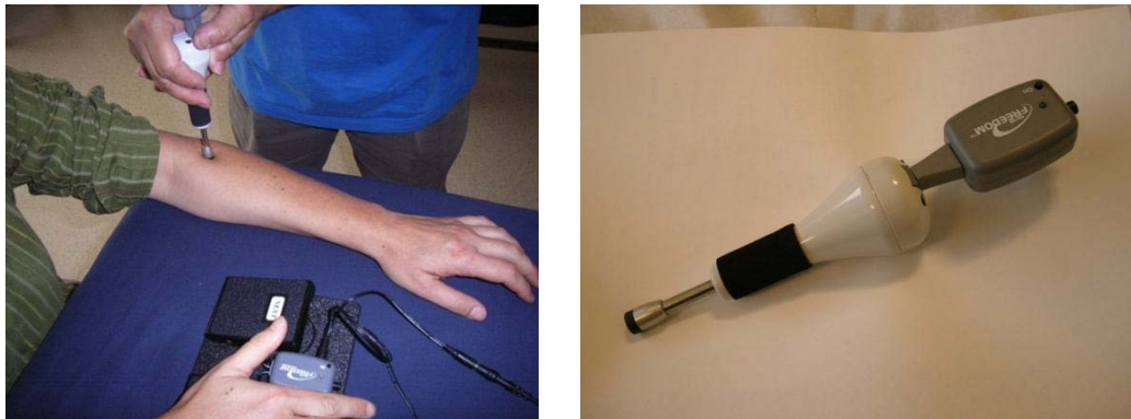
Figure 3.3: Left: Measuring PPT by an electronic algometer at LI10 of the left hand. The subject immediately pressed the pedal to record the data into the computerised system (Tracker Software Version 5) when the PPT was perceived. Right: The electronic algometer (Tracker Freedom ® ).
