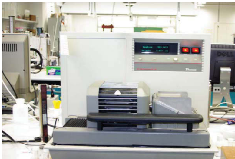
Figure 3-14 A TGA/DTA Analyzer (SDT 2960 model, TA Instruments) in UTS.
