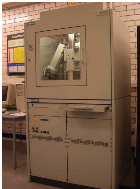
Figure 3-11 An X-ray diffractometer (Siemens D5000 model) in UTS.
