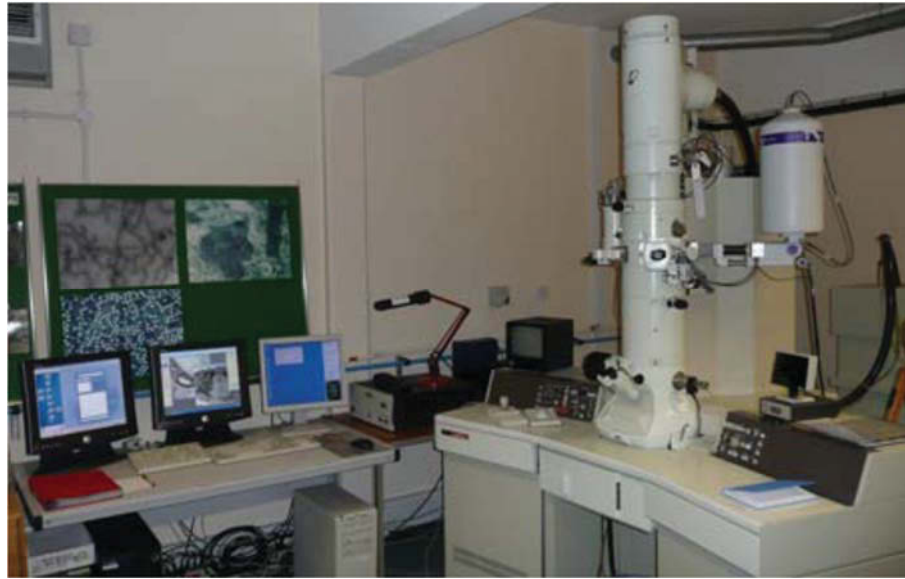
Figure 3-13 A commercial TEM setup (JEOL 2011 model).
