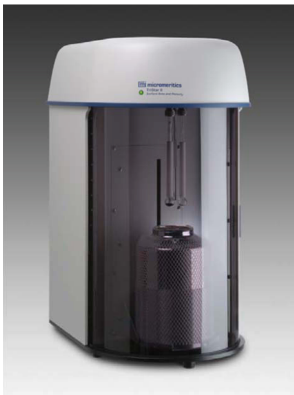
Figure 3-15 A TriStar II Surface Area Analyzer.
