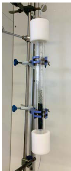
Figure 3.6 Small scale column with activated carbon and glass beads
