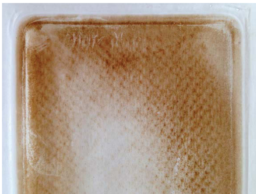
Figure 4.2.13 Fouled membrane with solution D containing 5 mg/L humic acid, 200 µg/L of each pesticide and the synthetic groundwater model solution.
