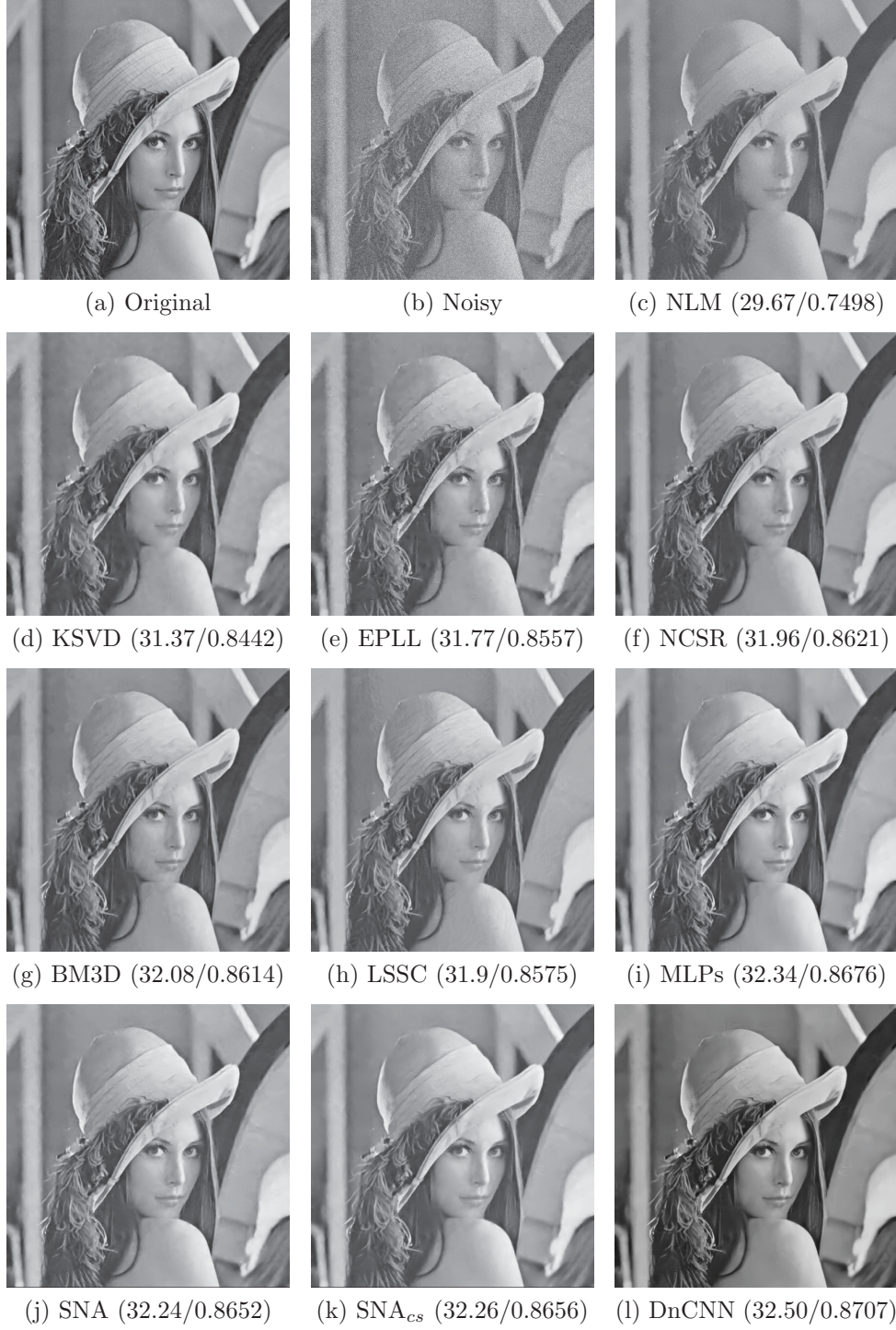
Figure 3.8: PSNR(dB) and SSIM results of different image denoising methods on lenna ( \sigma = 25 ).
