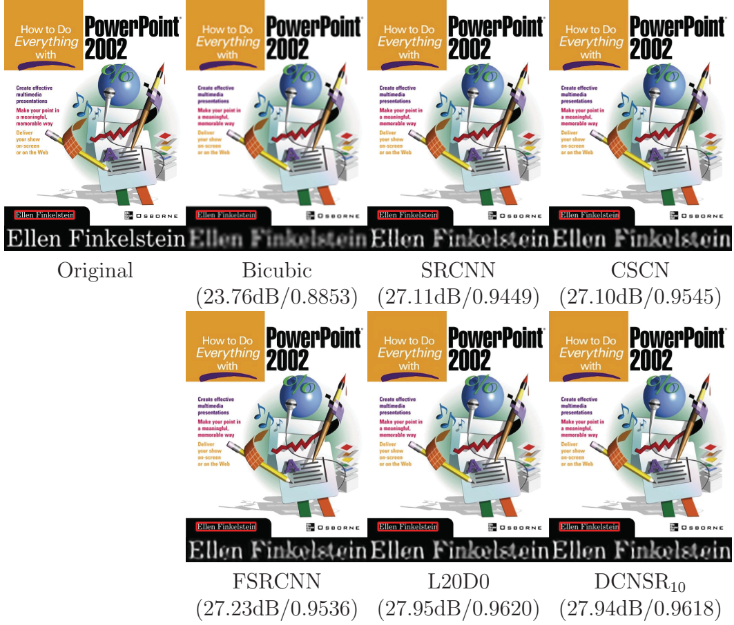
Figure 4.13: SR examples with an up-scaling factor of 3. PSNR/SSIM values are marked under each subfigure.
