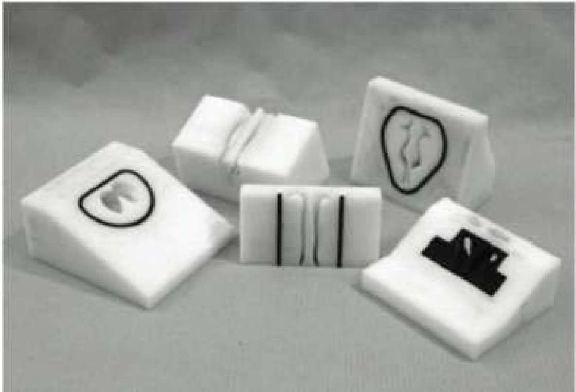
Figure 1.7. Part composing Boehringer-Ingelheim nasal Cast. Reproduced from reference [65] with permission
