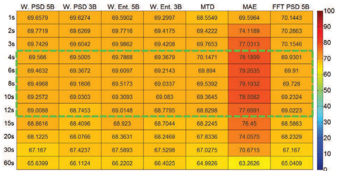
Figure 5.10: Suggested optimal window selection (OWS) color graph. The numbers in the graph reflect the weighted average accuracy of 4 emotions for each 7 features. The color heatmap expresses various levels of accuracy yield by window size between 1s and 60s for each of the 7 features, where darker colors represent higher accuracy. Referring to the graph, the optimal window can be identified.
