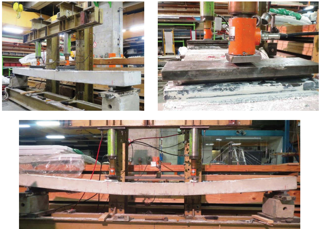
Figure 7.8: Load-deflection test setup and slab failure
