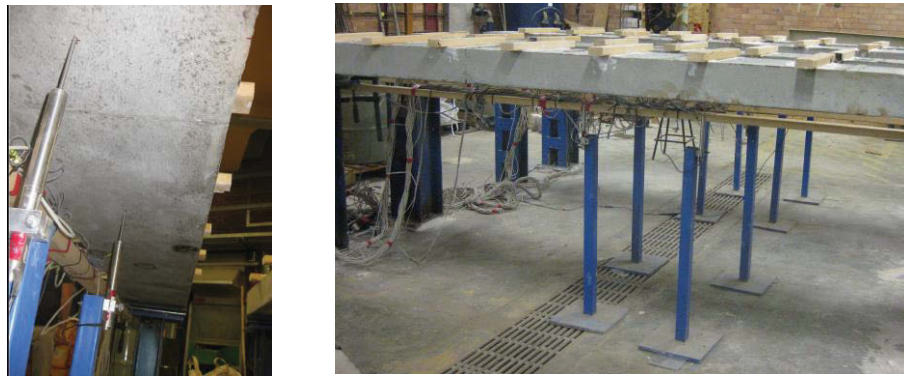
Figure 7.6: Installation of LVDT at two points of slab span
