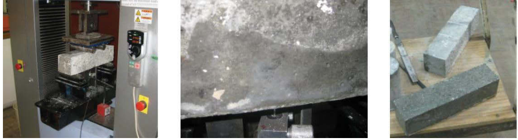
Figure 6.12: Specimen and testing equipment of flexural tensile strength
