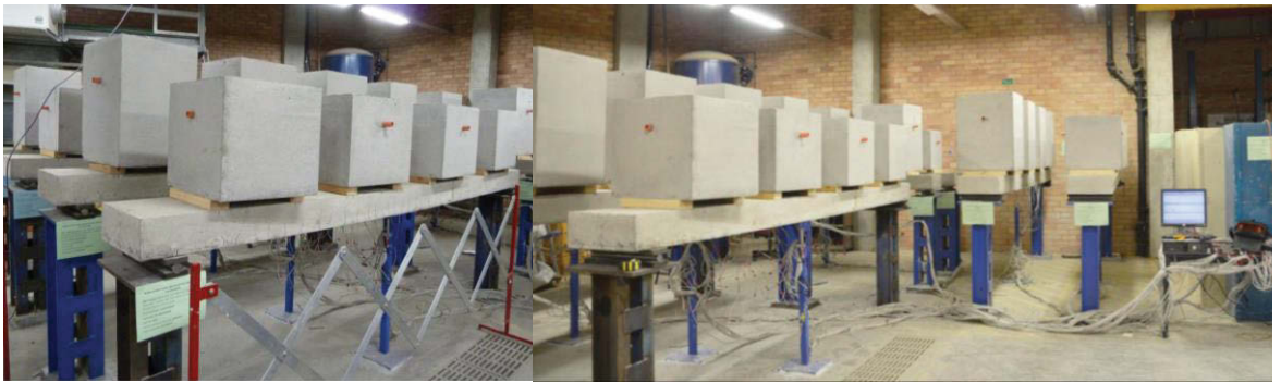
Figure 9.23: The loading of Self-compacting concrete slabs for time-dependent deflection monitoring (Aslani, 2014)
