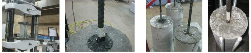
Figure 6.38: Pull-out test specimens and testing equipment
