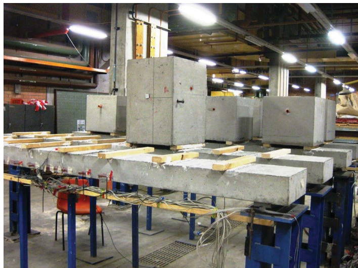
Figure 9.3: Loading pads and concrete block on the slabs for time-dependent testing
