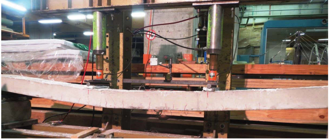
Figure 7.9: Deflection and cracking pattern of LWC-1 at failure point
