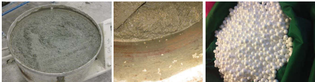
Figure 6.1: BST aggregates in fresh lightweight concrete
