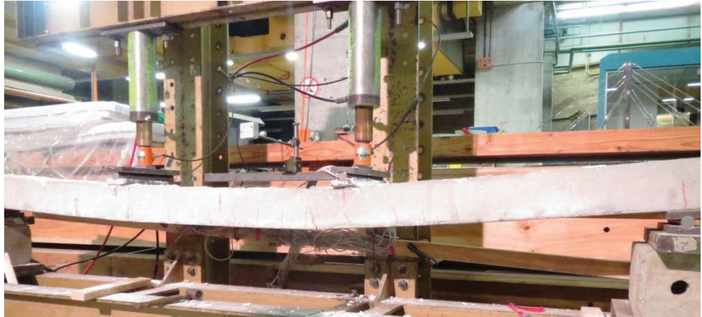
Figure 7.11: Deflection and cracking pattern of LWC-2 at failure point
