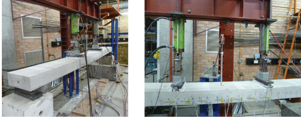
Figure 7.21: General view of the loading cells, concrete strain gauges and LVDT set-up [2]
