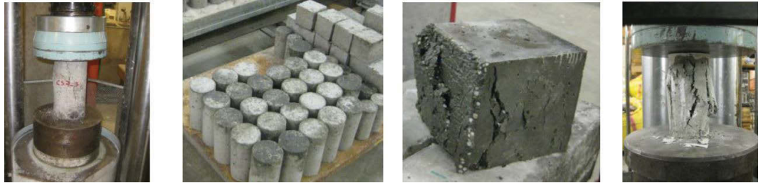
Figure 6.2: Testing setup and different sizes and shapes of the specimens for compressive strength tests
