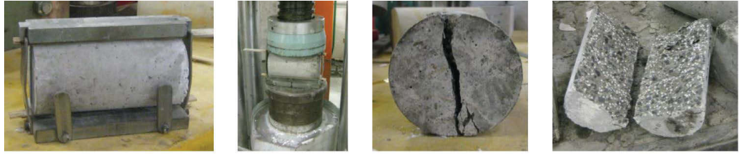
Figure 6.6: Specimen and test setup of splitting tensile strength
