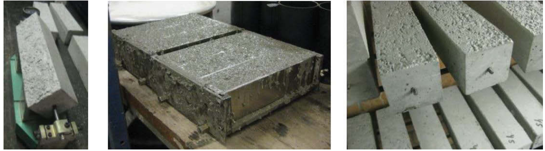
Figure 6.16: Shrinkage specimens and testing equipment
