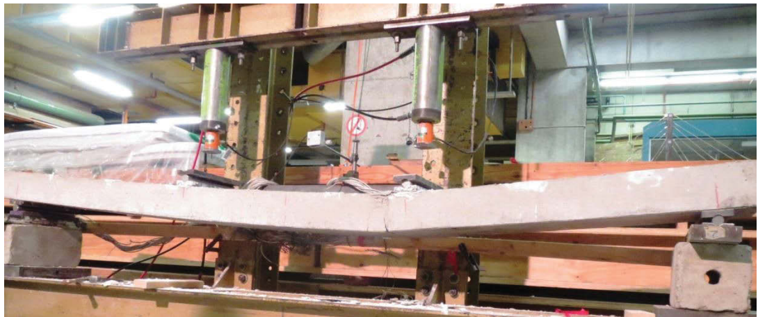
Figure 7.13: Deflection and cracking pattern of LWC-3 at failure point
