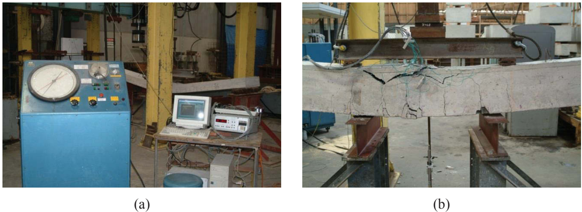
Figure 7.19: Failure of a) slab S2-b and b) beam B1-a [1]
