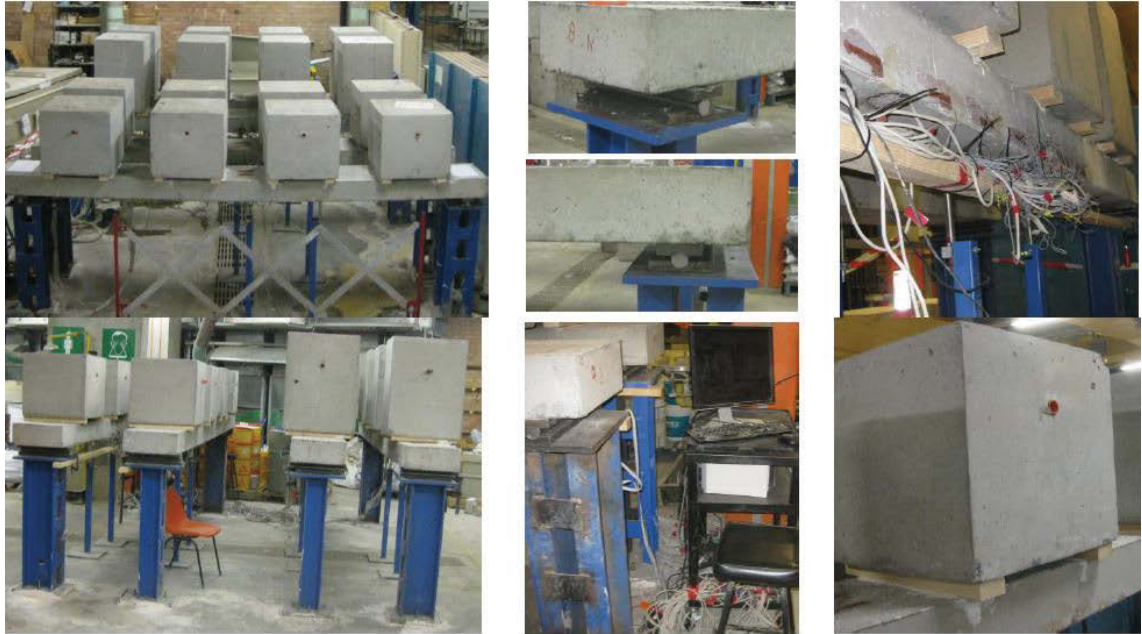
Figure 9.2: General view of the long-term deflection test set up of LWC slabs
