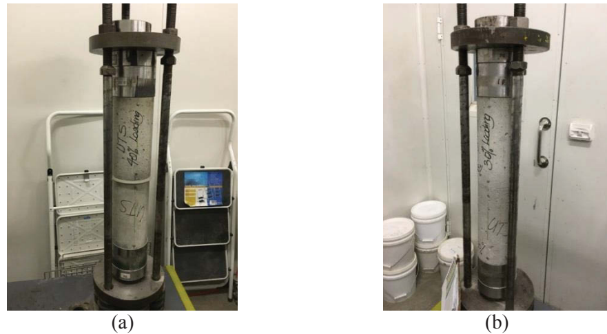
Figure 6.28: Creep test rig at two different loading levels
