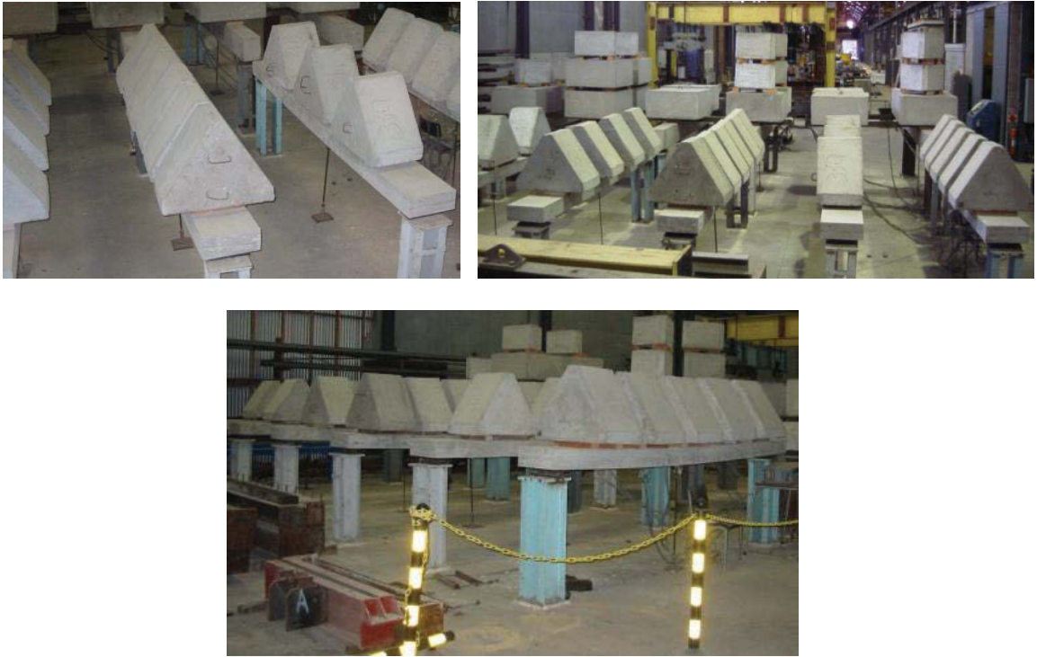
Figure 9.21: The loading of convention concrete slabs for time-dependent deflection monitoring
