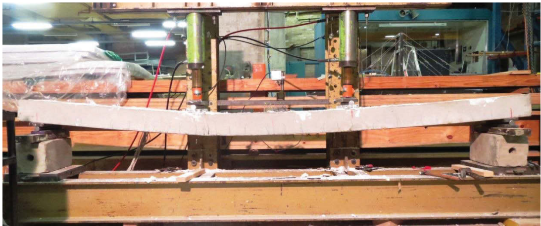
Figure 7.15: Deflection and cracking pattern of LWC-4 at failure point
