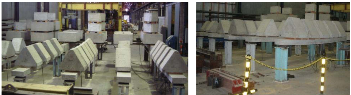
Figure 8.15: Loading of convention concrete slabs for time-dependent deflection monitoring (Nejadi, 2005)
