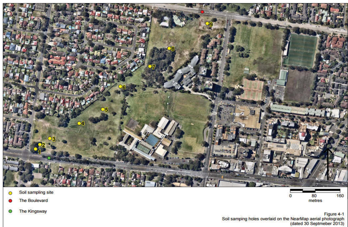
Figure 4-1 The initial transect conducted for preliminary analysis; the 9 yellow dots indicated the nine sampling locations for the trial test
