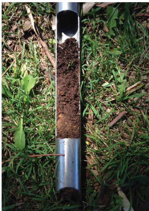
Figure 4-3 Stainless steel auger used for collection of samples
