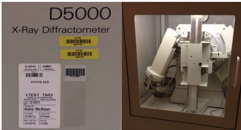
Figure 4-5 X-Ray Diffractometer, Siemens D-5000 used for soil mineralogy analysis
