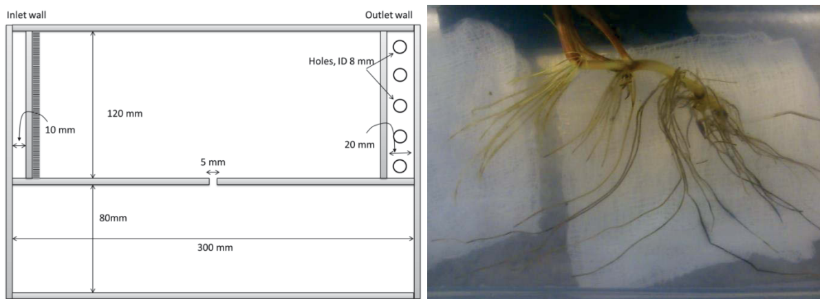
TOC figure. Left panel shows the design of the custom-made split flow chamber. Right panel shows the below-ground tissue embedded within the reduced, artificial sediment matrix.
