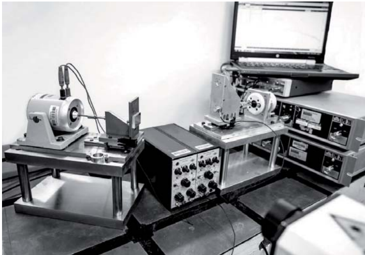
Figure 3: Experimental arrangement for 90° LDV to target surface/vibration direction scenario.
