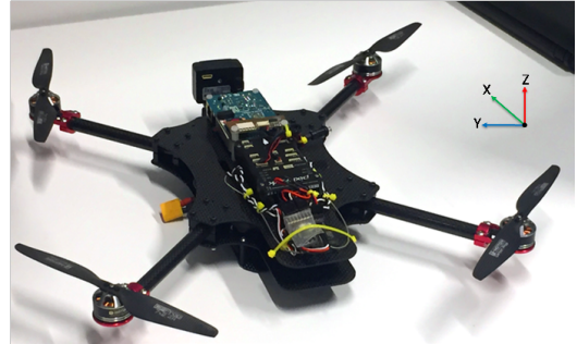
Figure 1: Proposed open-source multi-copter with autopilot, on-board computer and smart camera.
