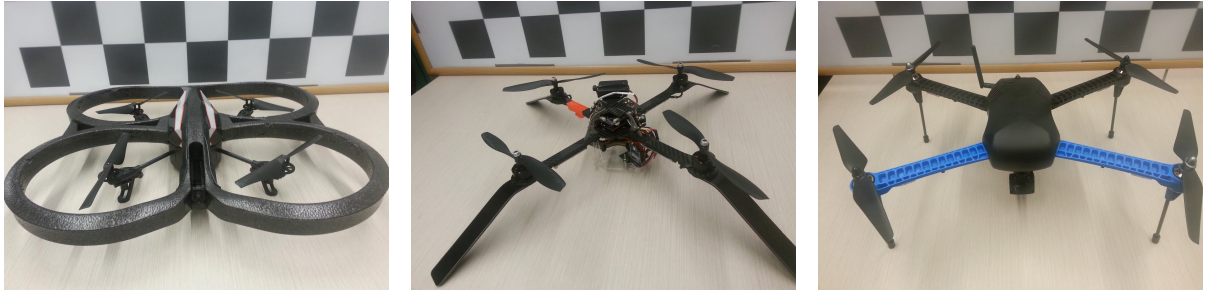
Figure 2: Common platforms: (a) Parrot AR Drone 2.0 (b) Ascending Technologies Hummingbird (c) 3D Robotics Iris+.
