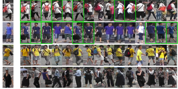
Figure 10: Sample re-ID results on the proposed PRW dataset with the DPM_Alex detector and the proposed IDE descriptor. Rows 1 and 2 are success cases, while Rows 3 and 4 are failure cases due to similar clothing and truncation, respectively. With truncated queries, partial re-ID methods [49] might be especially important.
