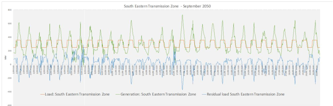
Figure 29 shows that generation in the south-eastern region exceeds demand and that power generation capacity is exported. To allocate generation capacity where demand is highest and therefore power grid infrastructure must cope with high loads makes economic sense. Load centers can therefore also operate as a ‘powerhouse’ for the region and/or country.
