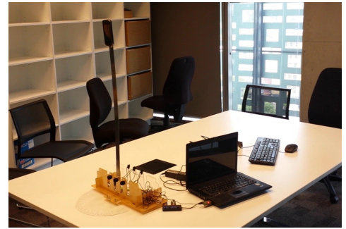
Fig. 9. Experimental setup of the asynchronous microphone array. Each channel of the array is sampled independently using individual USB sound card.
