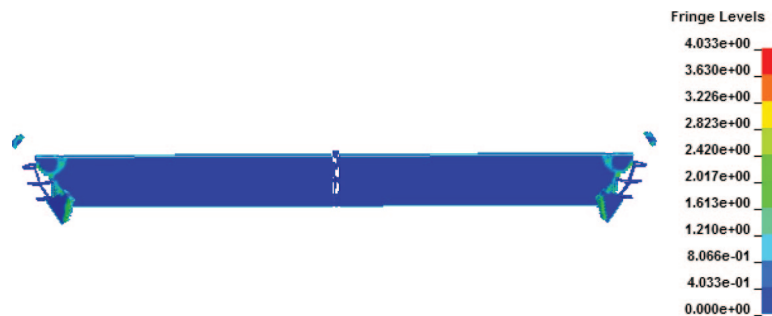
Figure 19. Failure mode of U1B column in the simulation
