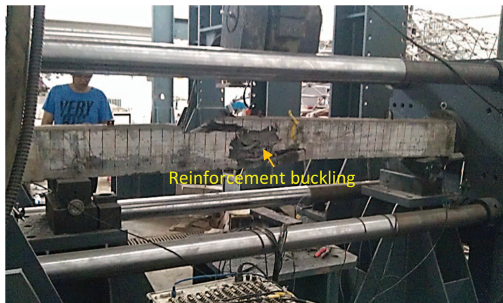
Figure 13. Failure of U2B column under residual load carrying capacity test
