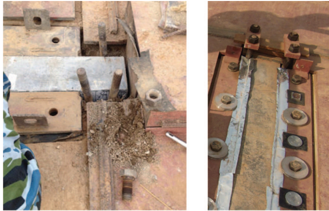
Figure 7. Column end boundary setup
