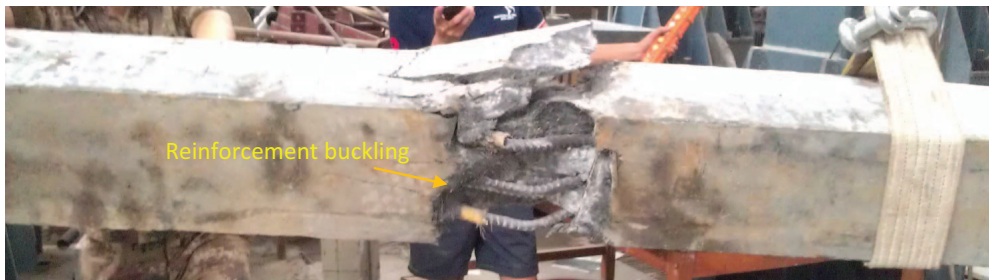
Figure 12. Failure of U1B column under residual load carrying capacity test
