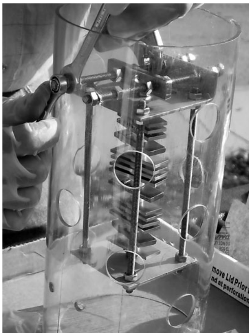
Fig. 5-3. Installing the test coupons in the coupon holder
