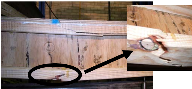
Figure 5: tensile failure of I-joist flange
