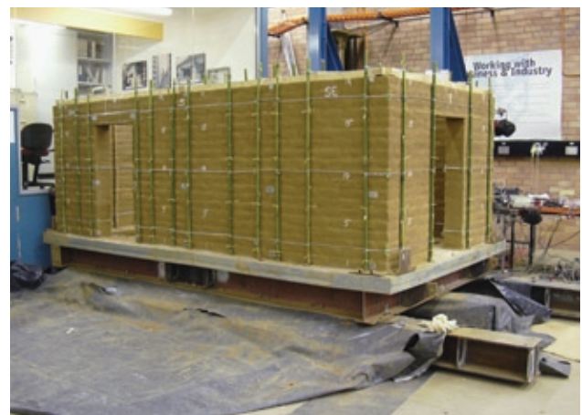
FIGURE 2 Model house 4A prior to testing; south and east walls are visible.
