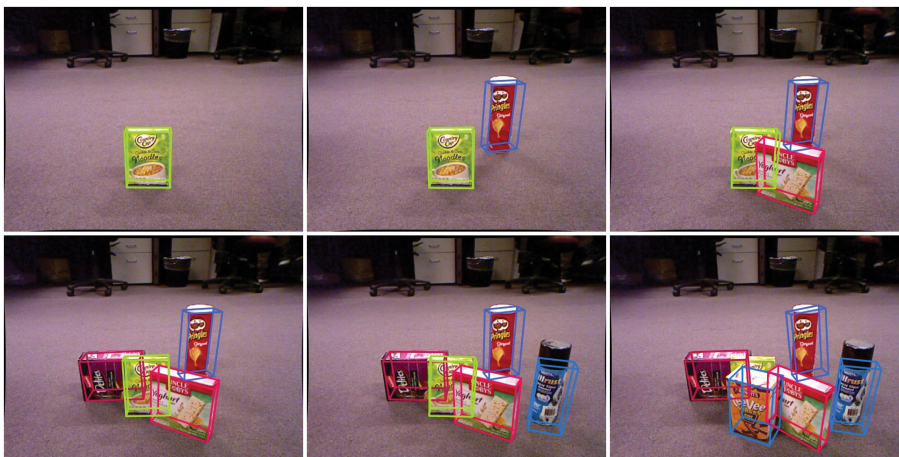
FIGURE 3.6: Objects detection and pose estimation results in cluttered environment.
