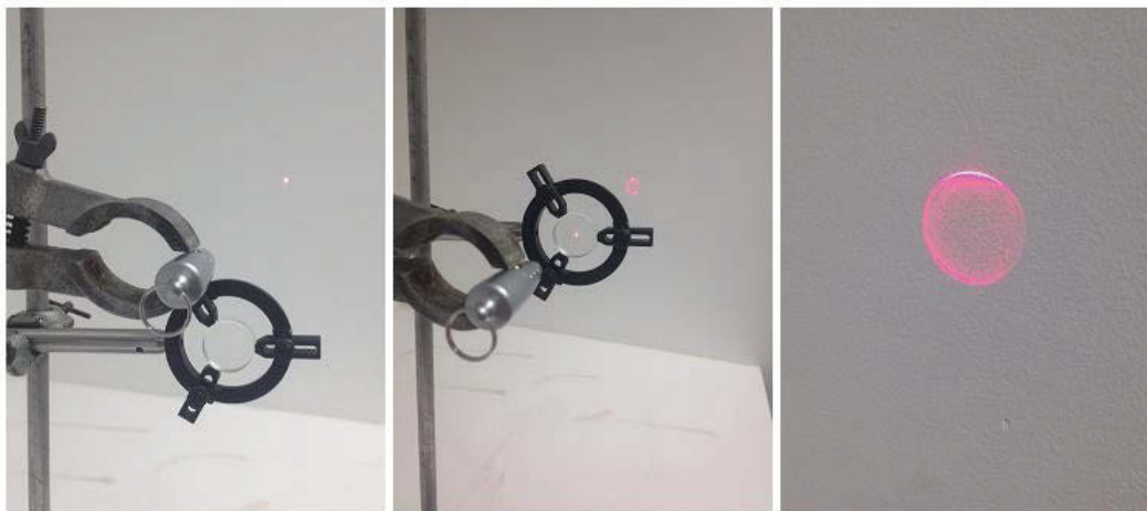
Figure 19 - Proof that the axicon used could facilitate the formation of a ring of laser light from a single point.
