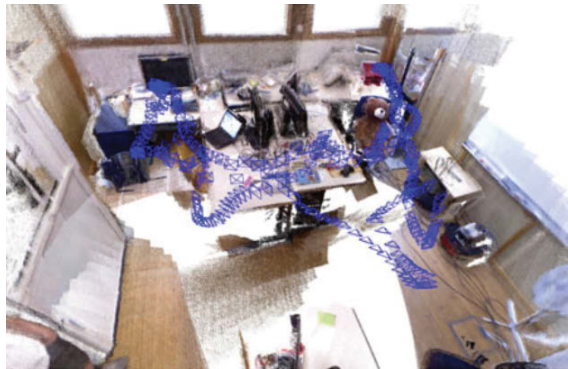
FIGURE 2.13: ORBSLAM2 with RGB-D input: Keyframes and dense pointcloud of a room scene with one loop closure [8].
