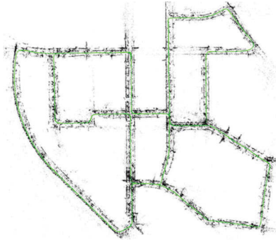
FIGURE 2.12: ORBSLAM2 with stereo input: Trajectory and sparse reconstruction of an urban environment with multiple loop closures [8].
