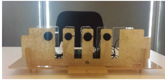
FIGURE 3.20: Experimental setup of the asynchronous microphone array.
