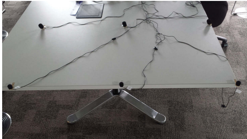
FIGURE 3.16: Experimental setup of the asynchronous microphone array. Each channel of the array is sampled independently using individual USB sound cards.
