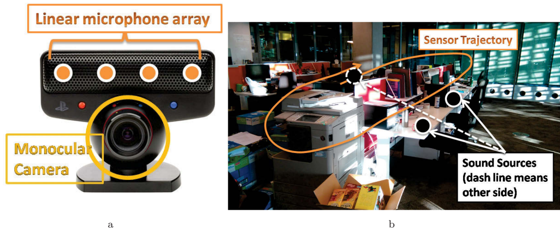
FIGURE 4.14: PS3-eye configuration (a) and experimental setup (b).
