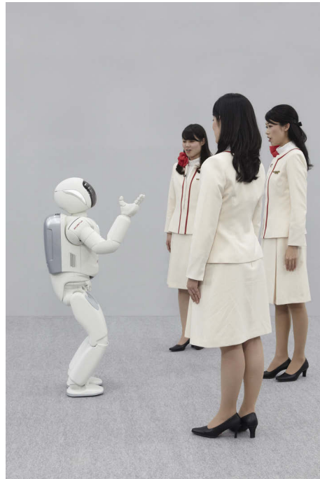
FIGURE 1.1: Asimo robot localises, separates and recognises simultaneous speech signals from three persons.
