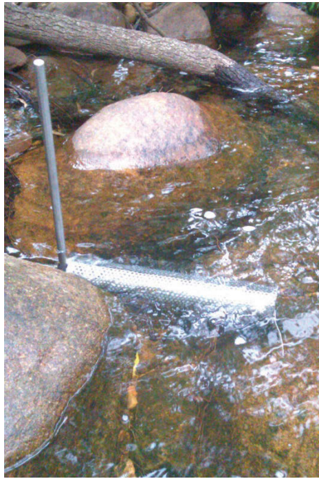
Supplementary Figure S5 a) an artificial substrate cage attached to the stream bed, b) view of the cage with removable glass slides on the detachable cage drawer insert.
