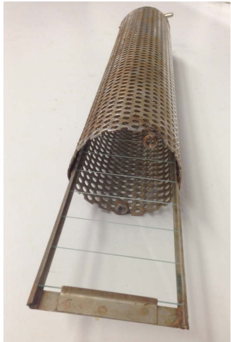
Supplementary Figure S5 a) an artificial substrate cage attached to the stream bed, b) view of the cage with removable glass slides on the detachable cage drawer insert.
