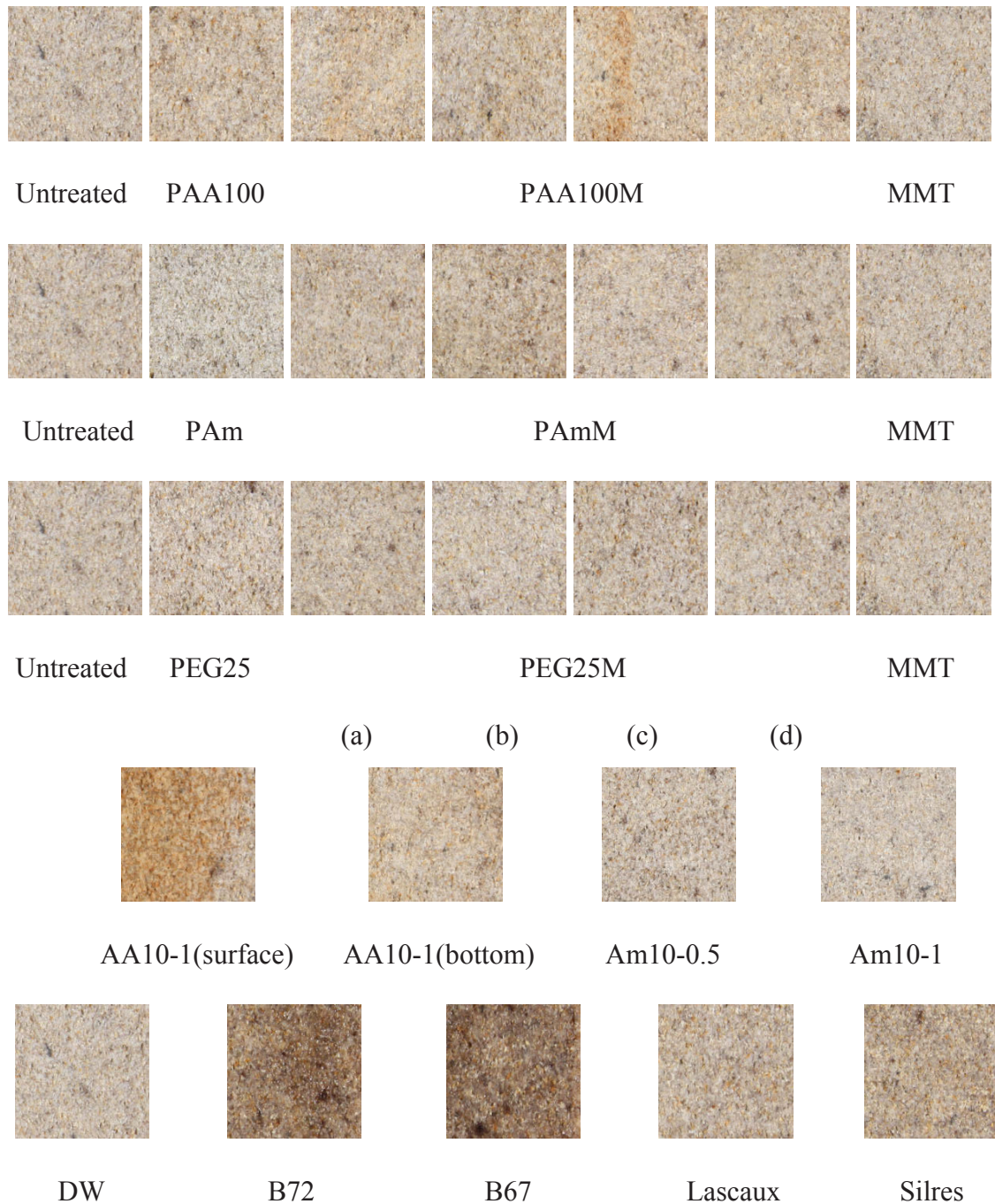
Figure 7.8.4. Images from immersed sections of sandstones treated with B72, B67, Lascaux, Silres, PAA100, PAm, PEG25 and polymer-MMT composites at (a) 20% MMT, (b) 40% MMT, (c) 60% MMT and (d) 80% MMT
