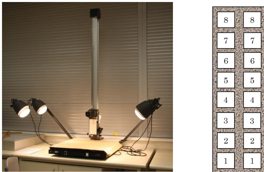
Figure 5.16. Polaroid MP-4 Multipurpose Camera Systems lighting stage with four 150W tungsten light bulbs angled at 45°(left) and order of colour sampling of sandstone specimens as processed in Photoshop CS5 (right)
