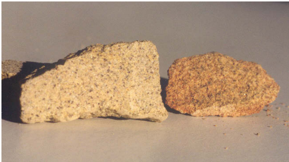
Figure 1.3. Unweathered (left) and discoloured (right) Sydney yellow block sandstone
