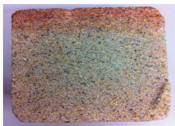
Figure 3.5. Photo image demonstrating the colour changes in the sandstone block as a result of weathering action on the uncovered surface to external environment
