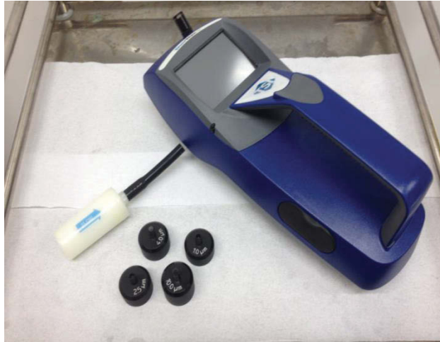
Figure 3.2 DustTrak II Handheld Aerosol Monitor (8532), a real-time aerosol mass readings device from TSI used for PM 10 and PM 2.5 concentration measurements.
