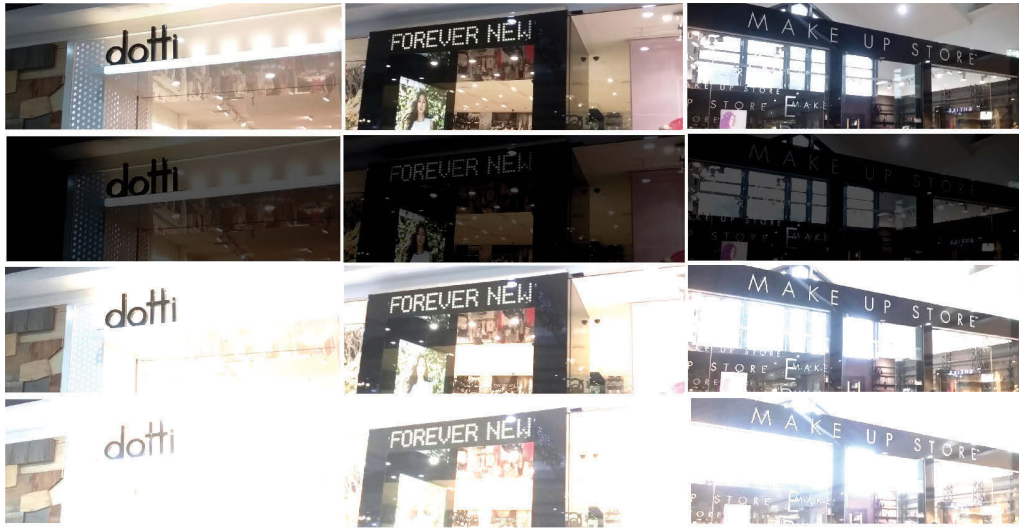
FIGURE 2.11: Test images with different illumination levels. Top row shows randomly selected three original test images, while second, third and fourth rows show same images modified with (\alpha = 0.5, \beta = -50) , (\alpha = 1.5, \beta = 50) and (\alpha = 2.0, \beta = 100) parameter values respectively.
