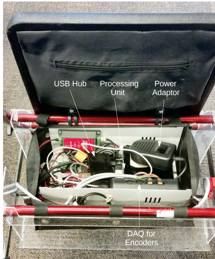
FIGURE 4.3: Experimental self-localization system placed inside walker container bag
