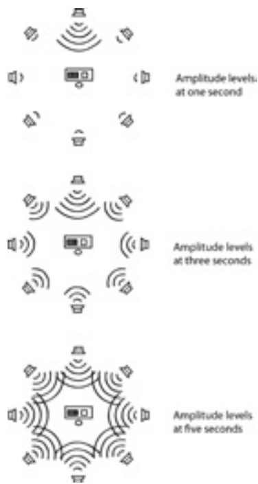
Figure 4. Amplitude point source panning [23] was used to create a sound diffusion for each spatial scene. This involved presenting a single sound source from the horizontal front centre loudspeaker. Over the duration of the first five seconds, sound sources were gradually presented from the remaining loudspeakers within a configuration.
