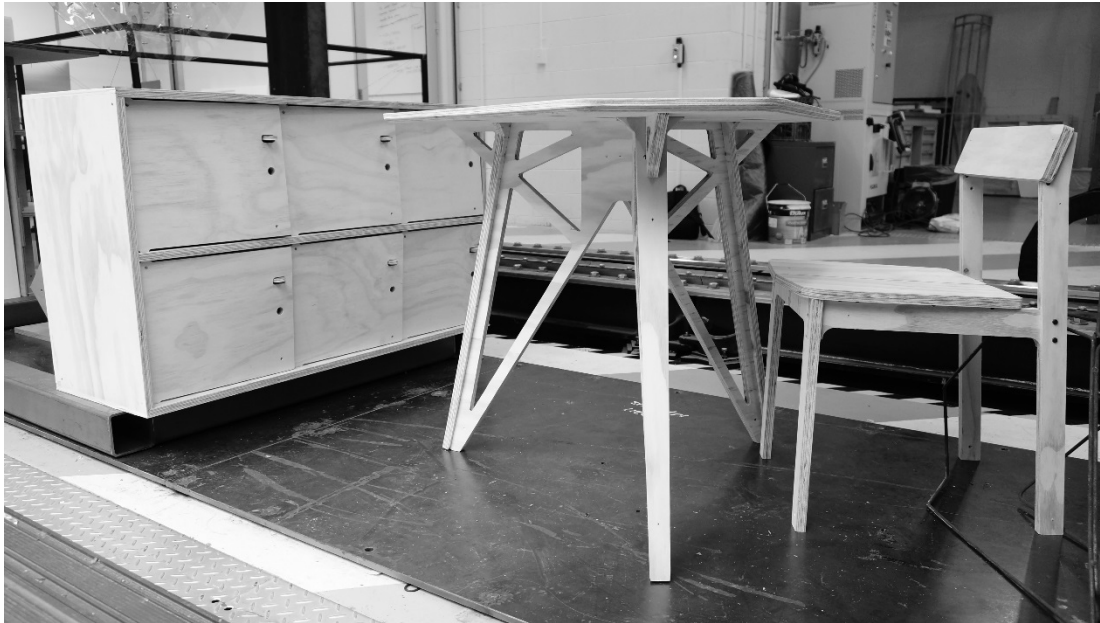
Figure 10: CNC made furniture by UTS using Open Desk designs (Finn Lockers; Half Sheet Table; Zero Pedestal)
