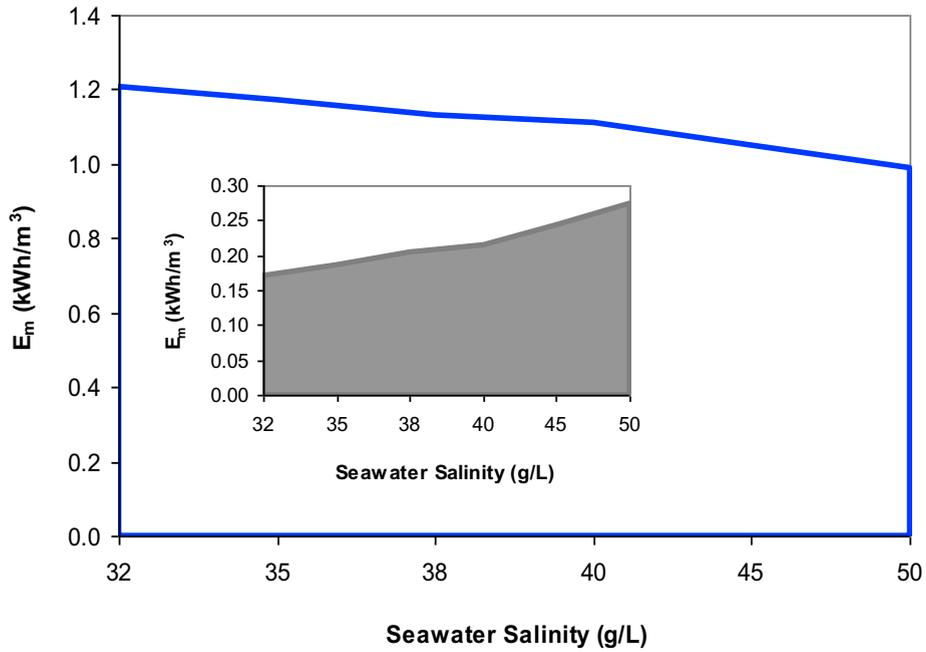
Figure 2: Maximum specific power generation from a number of salinity gradients made of coupling Dead Sea (DS) with seawater (SW) of salinities between 32 g/L and 50 g/L or coupling seawater (SW) with wastewater (WW).
