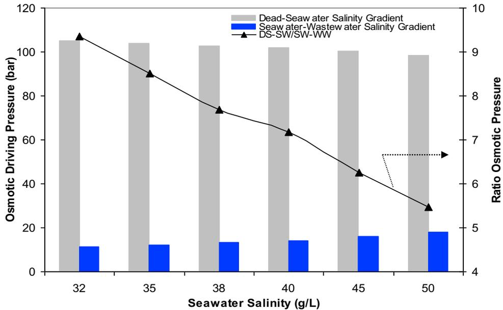
Figure 3: Osmotic driving pressure of different salinity gradient resources generated from coupling DS solution with seawater and seawater with wastewater
