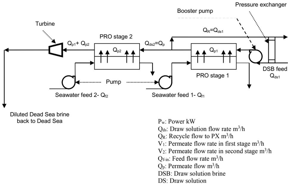
Figure 1: Schematic Diagram of Dual Stage PRO Process
