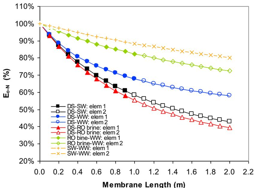
Figure 4: The specific energy along PRO modules in the pressure vessel. Dead Sea water (DS) is 5 M NaCl, RO brine is 1.2 M NaCl, seawater (SW) is 0.6 M NaCl, and wastewater (WW) is 0.017 M NaCl. The length of PRO module is 1.0 m and there are 2 modules in the pressure vessel.
