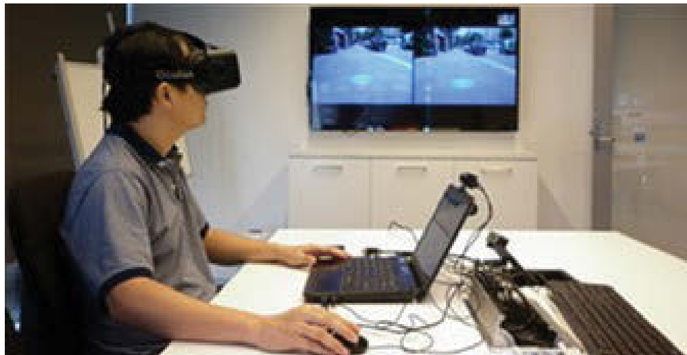
Figure 4.20: A remote user was wearing Oculus Rift and controlling the wheelchair in outdoor environments.
