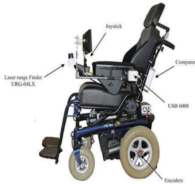
Figure 2.4: Intelligent wheelchair system (SAM), University of Technology Sydney, Australia, (Nguyen 2012).
