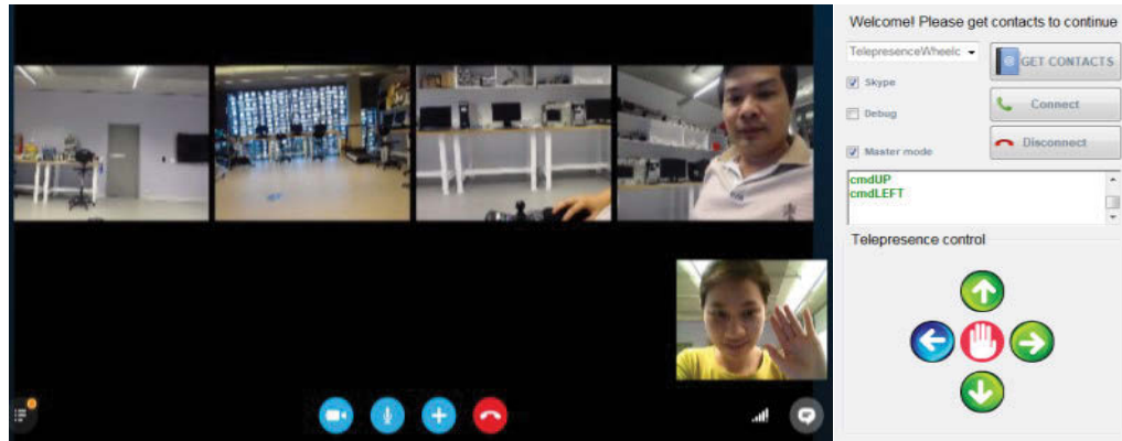
Figure 4.12: Multi-view video obtained from a telepresence wheelchair and the control interface at the remote site.
