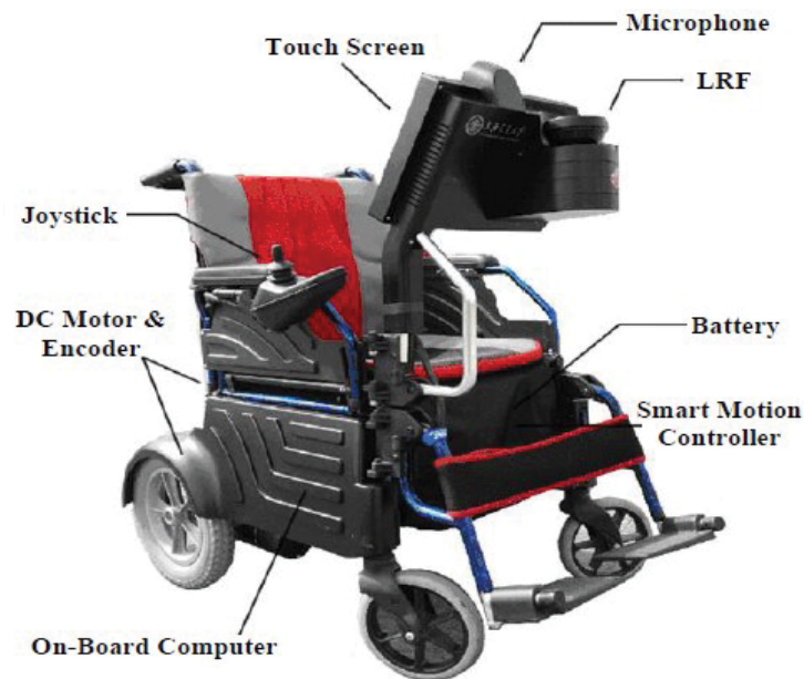
Figure 2.5: Intelligent wheelchair, Shanghai Jiao Tong University, China (Liu 2015).
