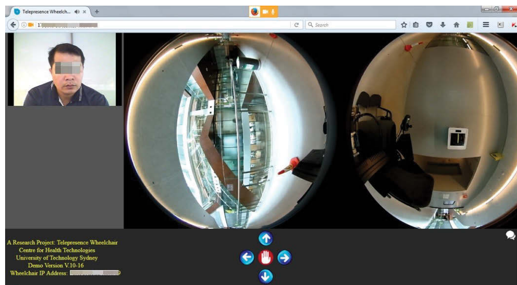
Figure 5.24: Dual-fisheye video without stitching processing.
