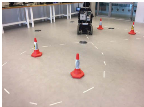
Figure 5.33: Test path setup with the figure eight curve.
