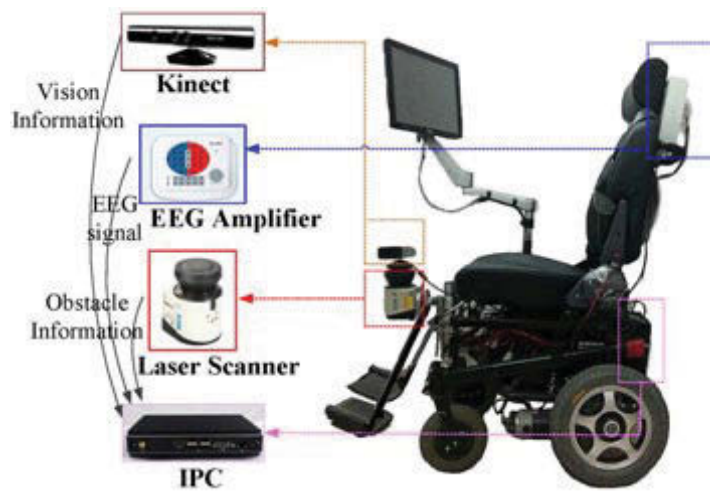
Figure 2.9: Brain-machine interface (BMI) wheelchair, (Li 2017).
