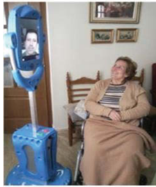
Figure 2.17: The Giraff telepresence robot, (Gonzalez 2012).
