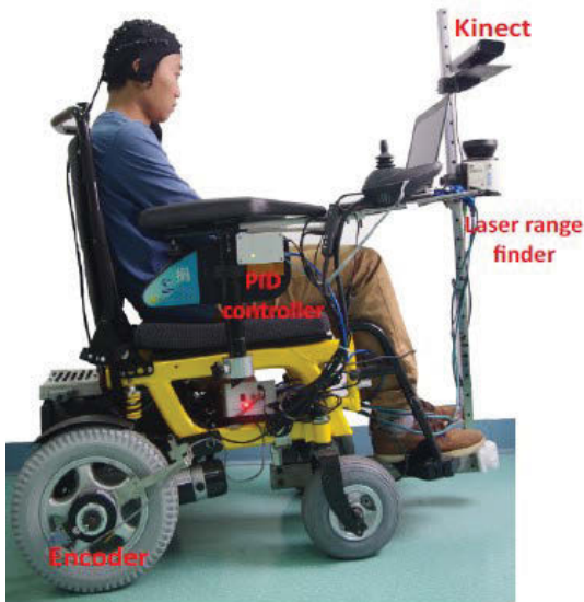
Figure 2.8: A BCI-based wheelchair, South China University of Technology, China, (Zhang 2016).
