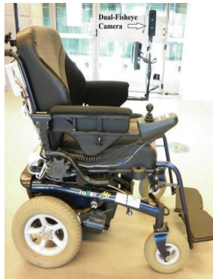
Figure 5.7: A telepresence wheelchair equipped with a dual-fisheye camera.
