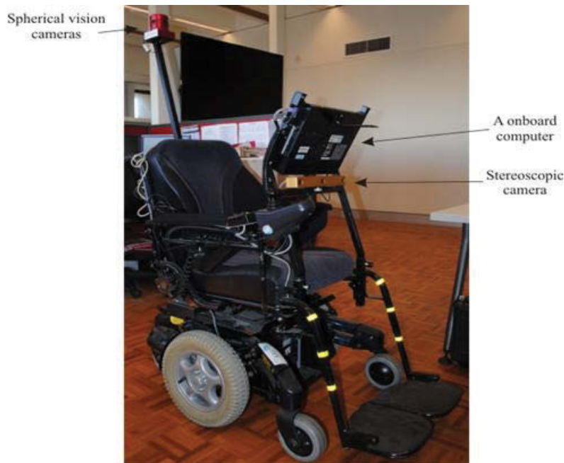
Figure 2.3: Smart wheelchair, University of Technology Sydney, (Nguyen 2013).
