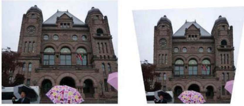
Fig. 10 – Perspective rectification of a building façade
