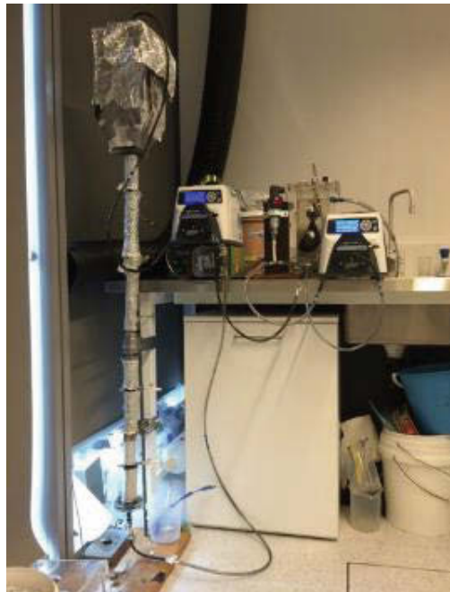
Figure 3.3 Experimental setup for preliminary G-AnMBR
