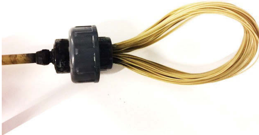
Figure 3.1 U-shape hollow fiber PVDF membrane module
