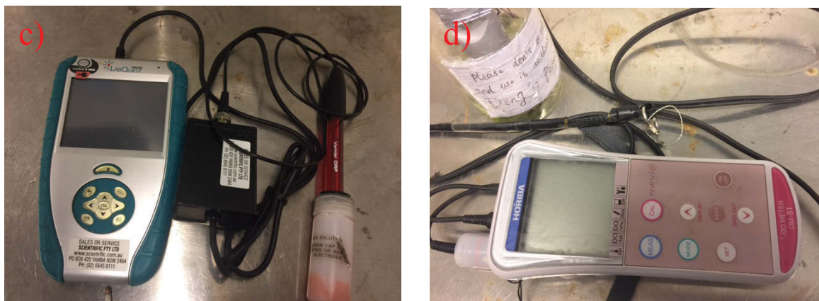
Figure 3.7 The analytical instruments used in the experimental investigation: a) DOC analyser; b) pH meter; c) ORP meter; d) DO meter
