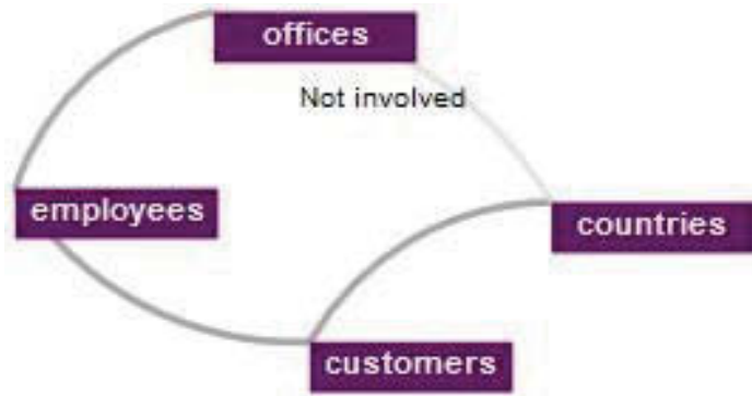
Figure 4.15 The instance of removing a link from a query. This query does not involve the relationship between offices and countries .
