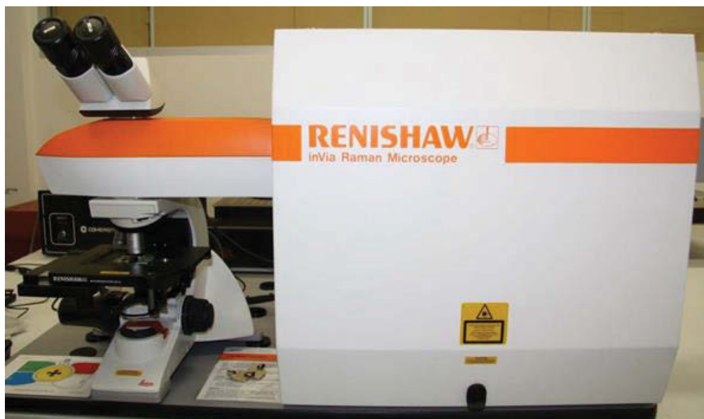
Figure 2-7 The Renishaw inVia Raman microscope equipped with a Leica DMLB microscope (Wetzlar, Germany) and a 17 mW at 633 nm Renishaw helium neon laser.
