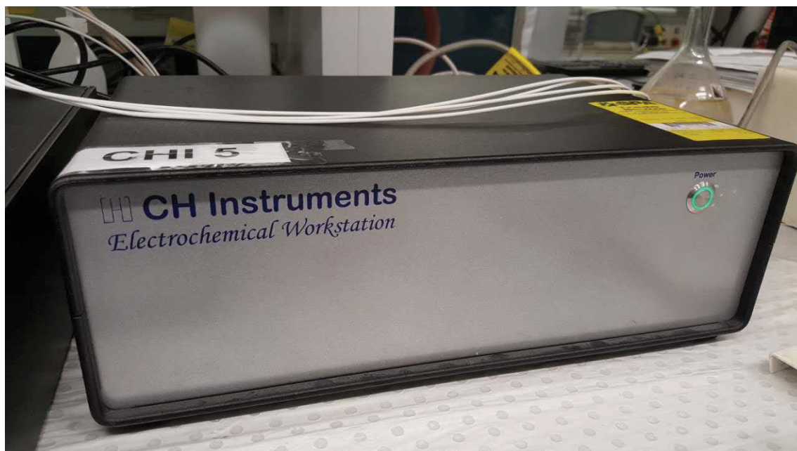
Figure 2-14 Photo of the CH instrument Electrochemical workstation
