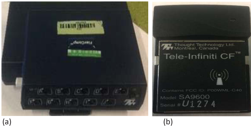
Figure 3.9 (a). Multichannel EMG Signal Encoder & (b). Compact Flash Signal transmitter
