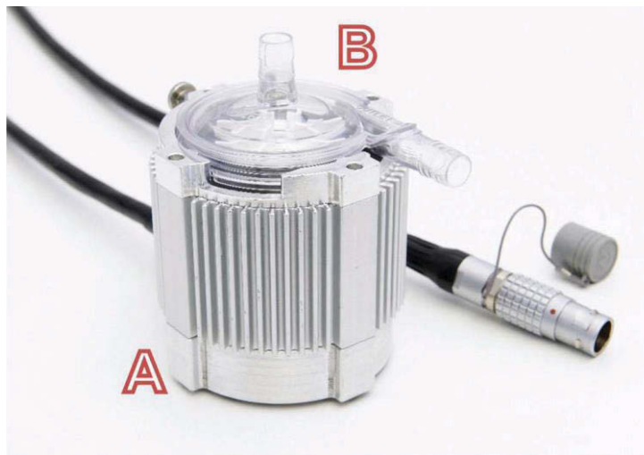
Figure 2.1 The Levitronix Cetrimag ventricular assist system. (A) bearingless magnetic motor. (B) Single use disposable pump head. (Courtesy of Thoratec Corporation)
