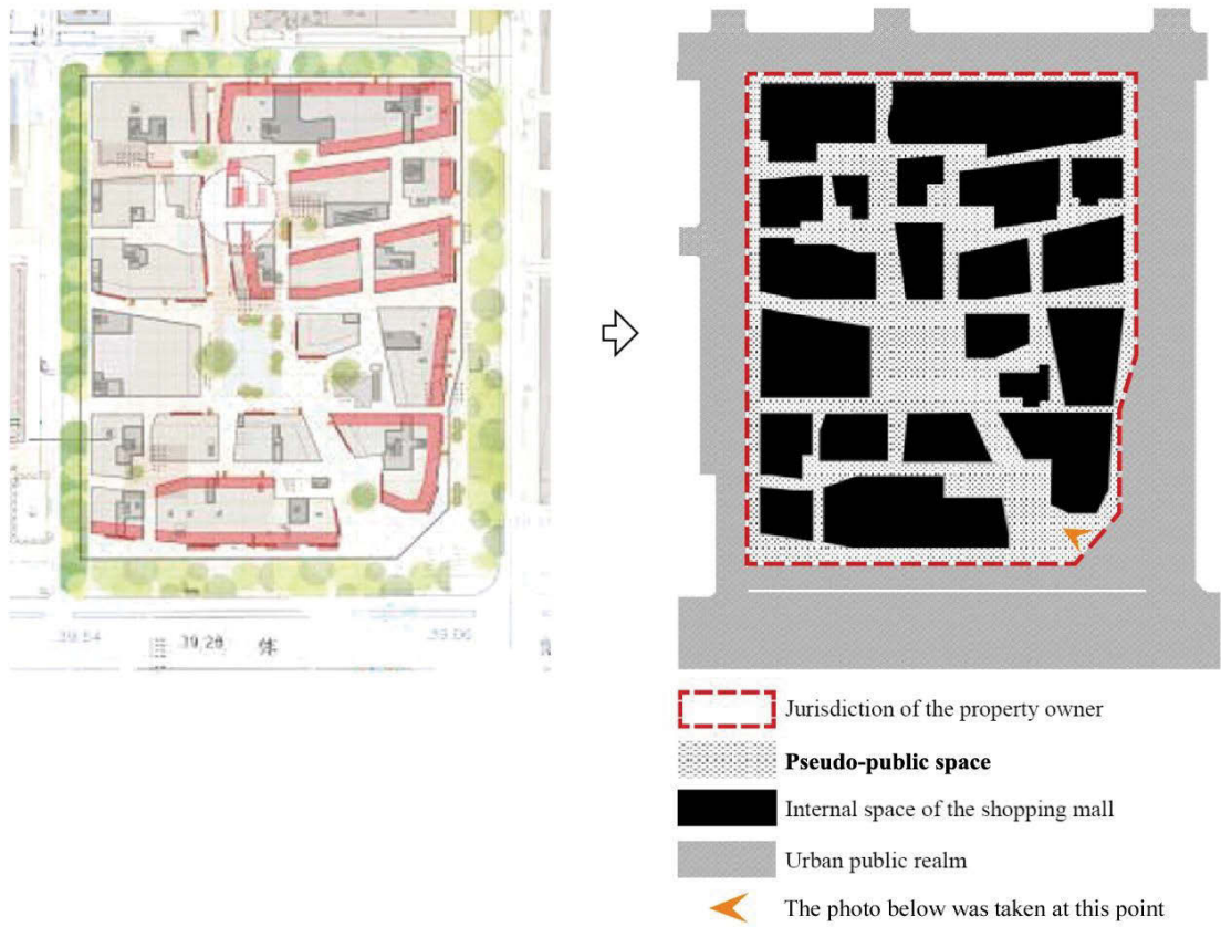
Fig 1.4 Sanlitun Village shopping mall in Beijing (below), its ground floor plan (left above), and a mapping of public realm, pseudo-public space, and internal space of the shopping mall in this urban area (right above)
