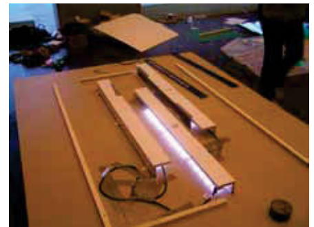
Figure 4.14 Plinth upside down showing ‘shelves’ for mounting LEDs
